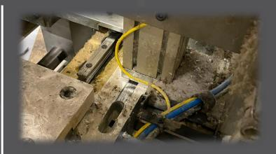
Missed daily cleaning resulting in excessive wear of a machine shaft
