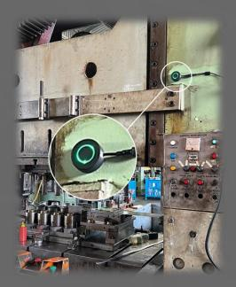
Non-invasive vibration sensor for asset condition and utilisation tracking
